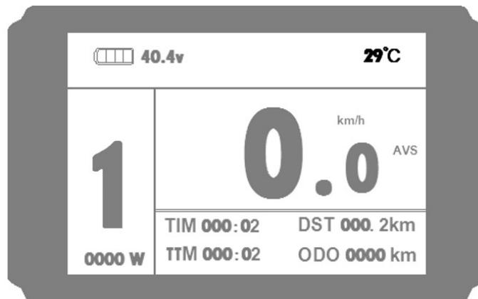
**The temperature display value may be in deviation shortly after boot-up, and the display value will be gradually approaching the environment temperature within 10 minutes after boot-up.**
