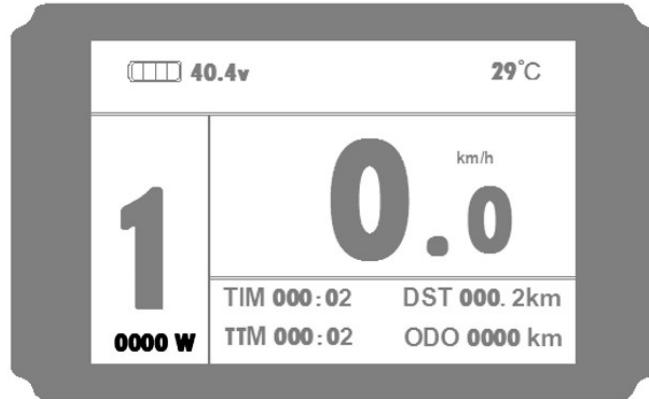
When C8 parameter setting is 1 (see C parameter setting), the meter turns on motor operating temperature display function.
